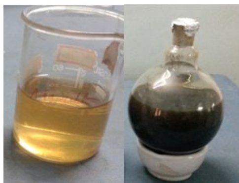
Figure 2: bio-reduction of silver nitrate using A. indica extract
