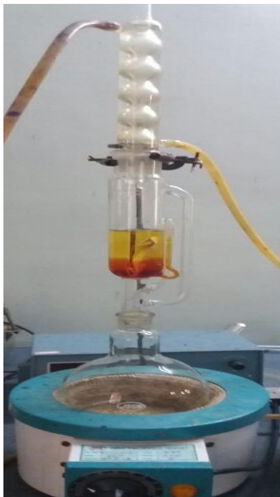
Figure 3: Soxhlet extraction of capsaicinoid from chilli samples
